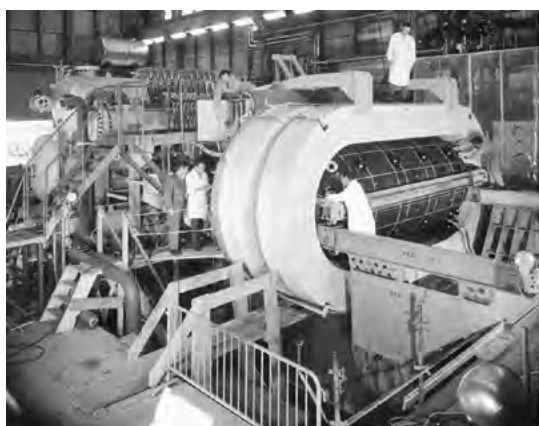
Figure 4: Picture of the Gargamelle bubble chamber and one of the neutral current candidates as observed in this experiment.
